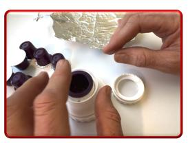
2. Fill a capsule with ground coffee and place it in Podpress as shown. It should sit nicely in the pocket, with its flange resting on the Podpress surface. If not, remove the capsule and make sure the surface is concentric and in uppermost position, centred and level with the top of Podpress' body.
