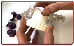
While holding the base, rotate the knurled Cap one complete turn. You should see the foil seal also rotate as you turn the cap. (in this action, Podpress is folding the foil under the capsule flange).
