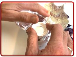
4. Put the Podpress cap over the foil around the centre of Podpress, and press down until you hear and feel a click and the cap is contacting Podpress body. In this process a circle of foil has been cut and separated from the sheet. 5. Grasping the Cap and Body together with one hand, with the other hand turn the knurled base anti-clockwise as far as it will go. This puts the capsule in position for the sealing process.
